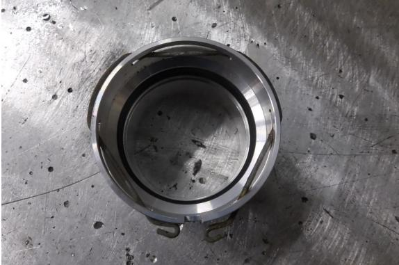
11. Fit the coupler to the intercooler, it is a tight fit so apply a good amount of pressure. You will know when it is seated correctly as you will hear an audible click as the retaining clip locks into position.
