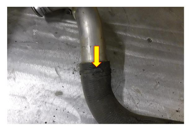
8. Using a 7mm socket and ratchet loosen the hose clamp attaching the noise generator hose to the plastic boost pipe. Now remove the hose from the vehicle.
