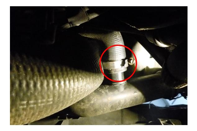
9. Using a 7mm socket and ratchet secure the first hose (#2099) from the FMKT035 kit to the plastic hard pipe with the supplied 30-45mm hose clamp.
