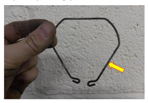
7. Using long nose pliers compress to loosen the hose clamp or alternatively use a hack saw or grinder to cut it off. You will now be able to remove the rubber hose from the hard pipe.
