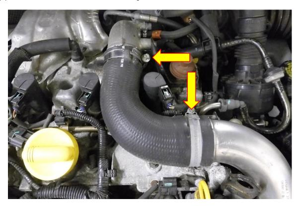
3. Again, using a 7mm socket and ratchet loosen the hose clamp attaching the noise generator hose. Next unclip the gearbox dipstick and using a 10mm spanner and ratchet remove the M6 fastener attaching the noise generator to the engine. The plastic part of the noise generator can now be removed.
