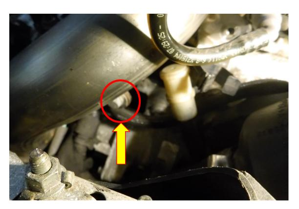
5. Using a ramp or a jack raise the vehicle in the air and support with axel stands if necessary, using a 10mm socket and ratchet remove all the X7 M8 fasteners. You will now be able to remove the undertray from the vehicle.
