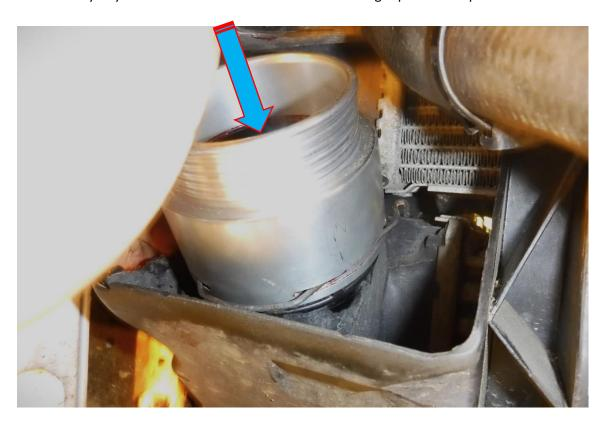
**12**. Using a 7mm socket and ratchet secure hose (#2101) to the coupler and the hard pipe using the supplied 50-70mm hose clamps.
