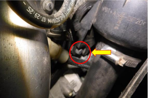
4. Using a 10mm socket and ratchet remove the X2 M6 fasteners attaching the hard pipe to the engine.
