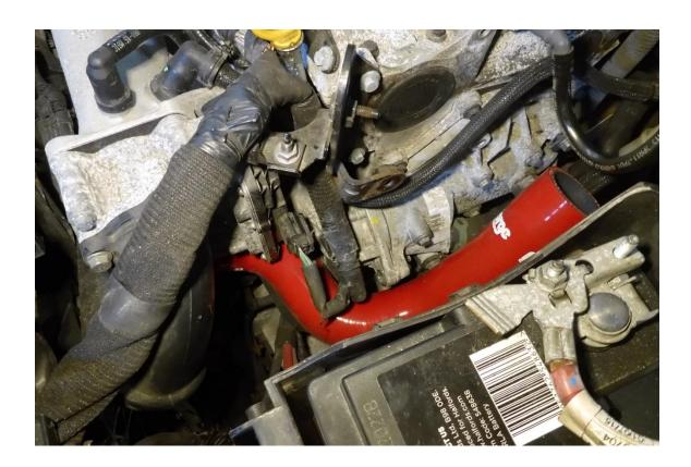
10. Take the coupler from the kit and smother it with grease or spray lubricant to help with installation. Now fit the retaining clip removed earlier in step 6 to the Forge coupler as shown in the second picture.
